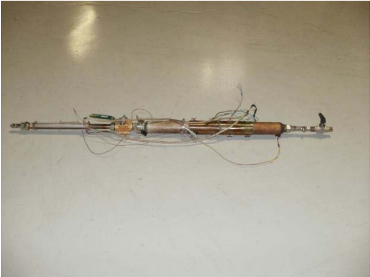
Figure 2-G-16.CVMR prototype carbonyl reactor.
