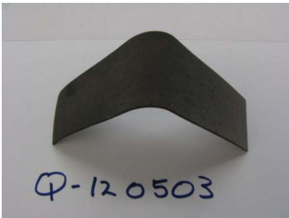
Figure 2-G-15. Bent carbonyl Ni-coated and annealed Zn alloy A190 strip.
