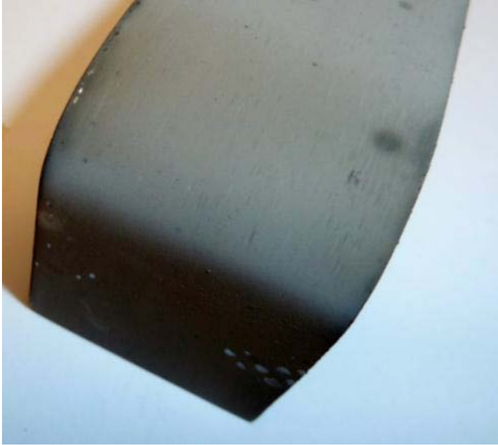
Figure 2-G-11. Carbonyl nickel-coated steel specimen after single-bend testing.
